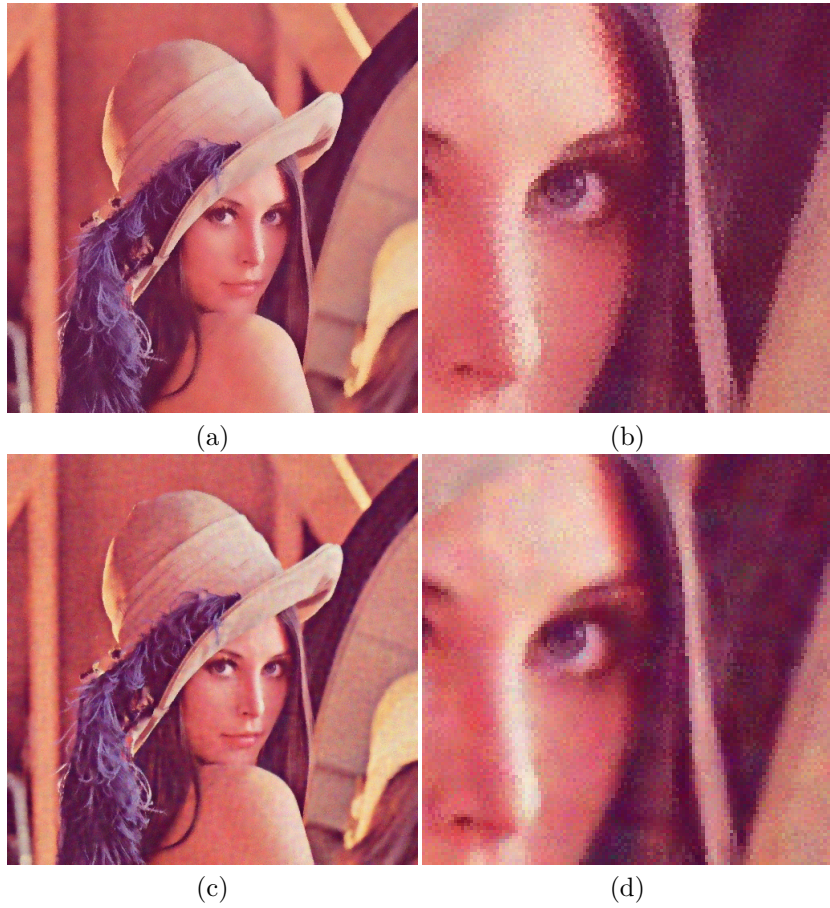
Figure 12: Denoising (Gaussian Noise) on Color Image: (a) and (b): Bilateral KR ( N = 0 , window size = 11, h_s = 100.0 , h_d = 0.1 ). Error: 0.039308 (RMSE) and 28.1104 dB (SNR), (c) and (d): Bilateral KR ( N = 2 , window size = 11, h_s = 100.0 , h_d = 0.1 ). Error: 0.038411 (RMSE) and 28.311 dB (SNR).
