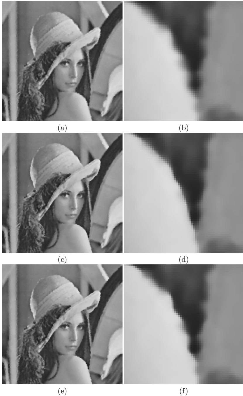
Figure 8: Reconstruction: (a) and (b): Linear KR ( N = 0 , window size = 11, h_s = 2.0 ). RMSE (comparison with ground truth): 0.043029, (c) and (d): Bilateral KR ( N = 0 , window size = 11, h_s = 2.0 , h_d = 0.4 ). RMSE (comparison with ground truth): 0.037698, (e) and (f): Robust KR ( N = 0 , window size = 11, h_s = 2.0 , h_r = 0.4 , number of iterations = 5). RMSE (comparison with ground truth): 0.041621.
