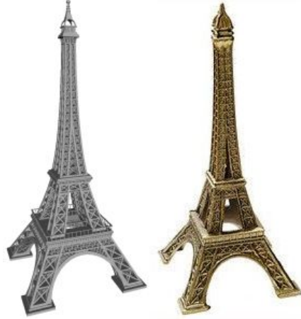
Figure 7.1.1: Rendering vs. Manufacturing 3D models capturing every hole and protrusion of real-world objects (left) render correctly at any far camera view. We draw inspiration from souvenir manufacturing where detail is manually abstracted and engraved to ensure that miniature models are fabricatable (right).
