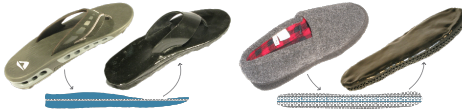
Figure 5.0.1: Physically Replicating Deformation Behavior Given the deformation behavior of real world objects in form of measured example deformations, we estimate layered approximate models, tailored for 3D manufacturing using multi-material AM technologies. Our replicas' deformation properties are in high agreement with those of the input.
