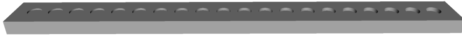
Figure 7.3.1: Calibrating Engraving Depth We designed a part with cylindrical intrusions of varying depths to identify the minimal engraving depth for a particular printer-material pair.
