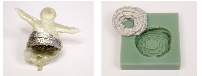
Figure 5: Dual-material optimization: (Left) dual-material model, (right) 3D printed mold and resulting metal cast.
