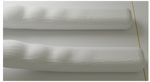
Figure 9: Showcase of the worm optimization. The baseline robot is on the top while the optimized one is at the bottom. This was taken after 6 seconds, or double the optimization end time.
