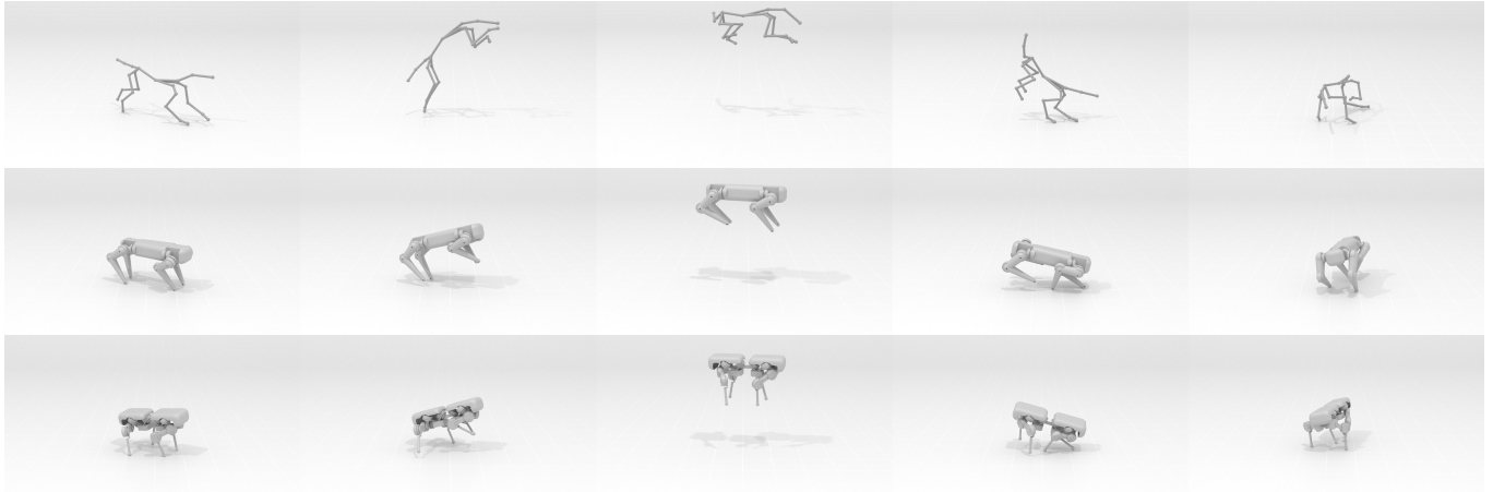
Fig. 6. Retargeting of mocap motion M1 onto Max and Lizard robots. Top row shows the skeleton motion input, for representative frames. Middle row shows the result on Max; bottom row shows the result on Lizard. Despite the differences in kinematics between the input and the two robots, the characteristic traits of the motion are preserved. (Mirrored w.r.t. video.)
