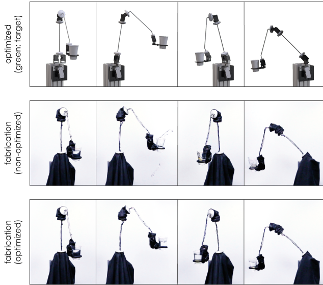
Fig. 11. Bartender Robot. The top row shows 4 frames of the simulated optimization result while the middle row shows the physical robot executing the non-optimized trajectory and spilling the drink (frames 2 and 4). Bottom row shows corresponding frames from the optimized trajectory, with no spillage.
