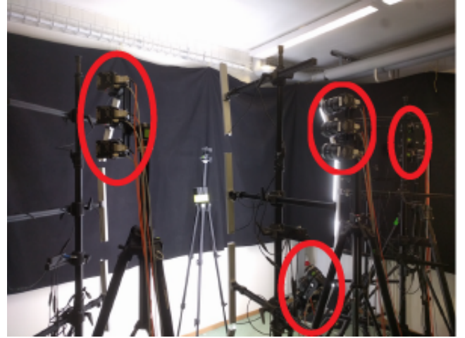
Figure 3: Capture setup with four stereo cameras pairs and a tripod standing in for an actor.
