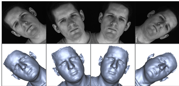
Figure 4: Here we show a subset of the captured performance. The actor tilts his head to each side, providing different tissue deformation due to the known gravitational force.
