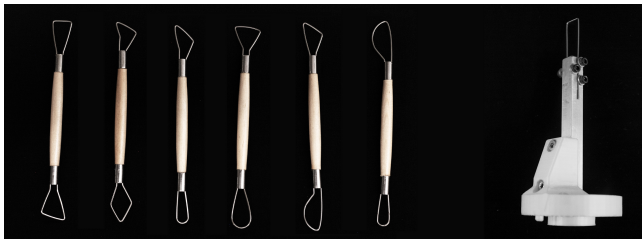
Figure 3: Left: different manual loop tools used by professional sculptors; Right: our customized loop tool that can be attached to a UR5 as the robot end effector.
