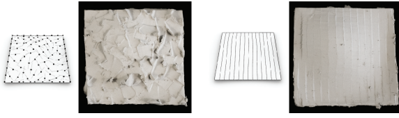
Figure 5: Left: surface sculpted with 100 toolpaths of 18 mm length in random direction, generated from 100 randomly sampled points; Right: the same surface sculpted with 15 parallel toolpaths across the whole width of the patch.
