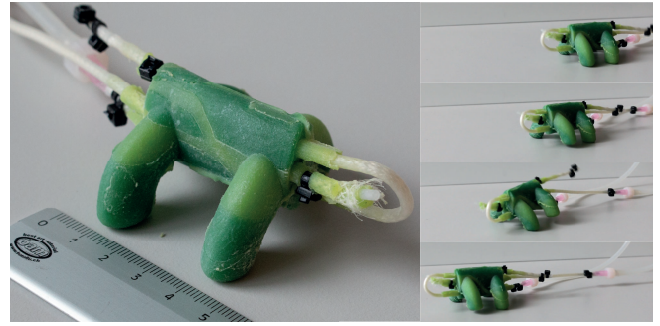
Fig. 16. Walking robot, experiment. The body length of the robot is 42 mm. The robot achieves a forward velocity of 7.9 body lengths/min. See also the supporting video. The two colors on the robot body come from the two-step molding process, see Fig. 7.
