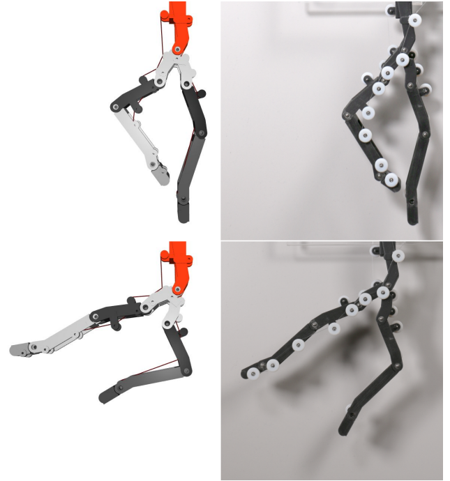
Figure 11: We validate our cable network optimization on the lower body of our Fighter character on two target poses (bottom, top) by controlling the cable forces with standard Newton meters. The simulated poses (left) match the physical poses (right) well.
