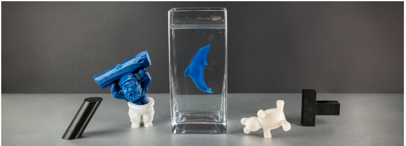
Figure 1: (From left to right) The Sheared Cylinder , the Muscle Gnome , the Dolphin , the Breakdancing Teddy , and the T Shape are all models whose complex balance is made possible by using movable masses and optimization with our method.
